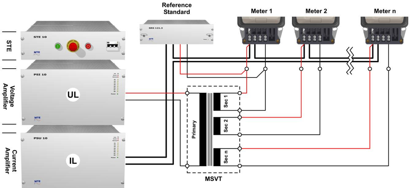
If multi-tariff meters are to be tested, the energising voltages for the tariff relays also must be galvanically isolated. In this case the voltage transformer requires the addition of a relay with a separate
