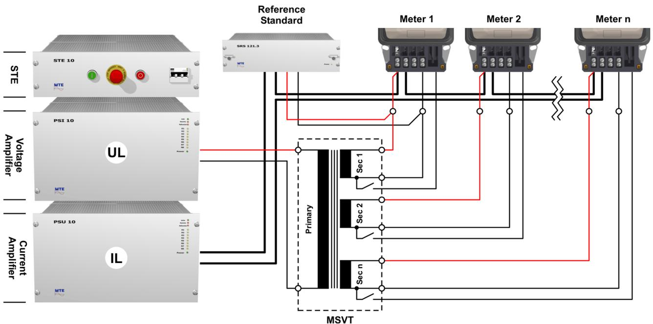
As with most high accuracy voltage transformers, these MSIVTs are specified for only one nominal voltage.
